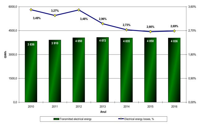
Figure 2.23 The evolution of the total electrical energy losses in RET.
