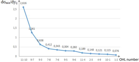
Figure 2.29 Partial derivatives of Jacobian's minimal singular value with respect to the admittances of the electric power system's single line diagram elements
