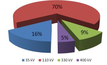
Figure 2.10 The rate of TSO's OHLs at different nominal voltages
