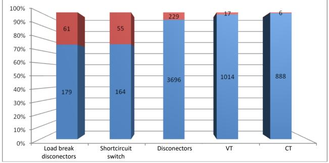
Figure 2.9 TSO's electrical equipment technical state
