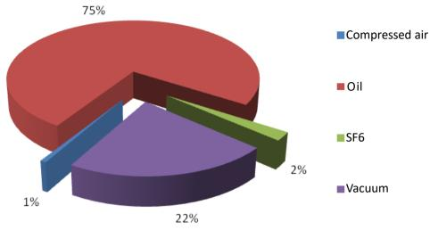
Figure 2.7 The rate of the 10-400 kV TSO's circuit breakers
