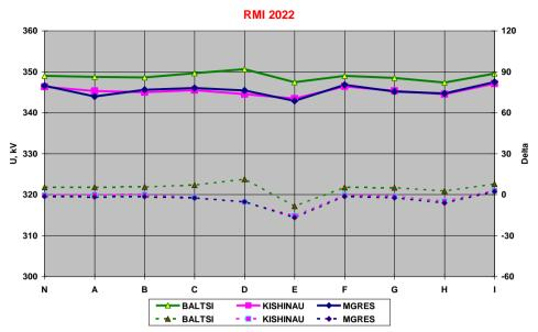
Figure 4.3 Voltages and angles in transmission grid nodes, with N-1 elements in operation, for calculation model for year 2022
