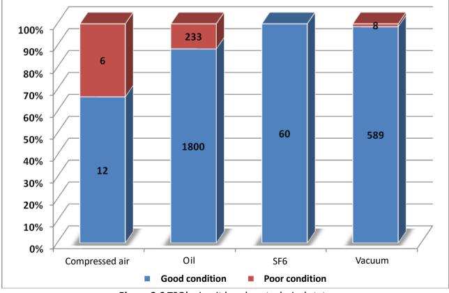
Figure 2.6 TSO's circuit breakers technical state
